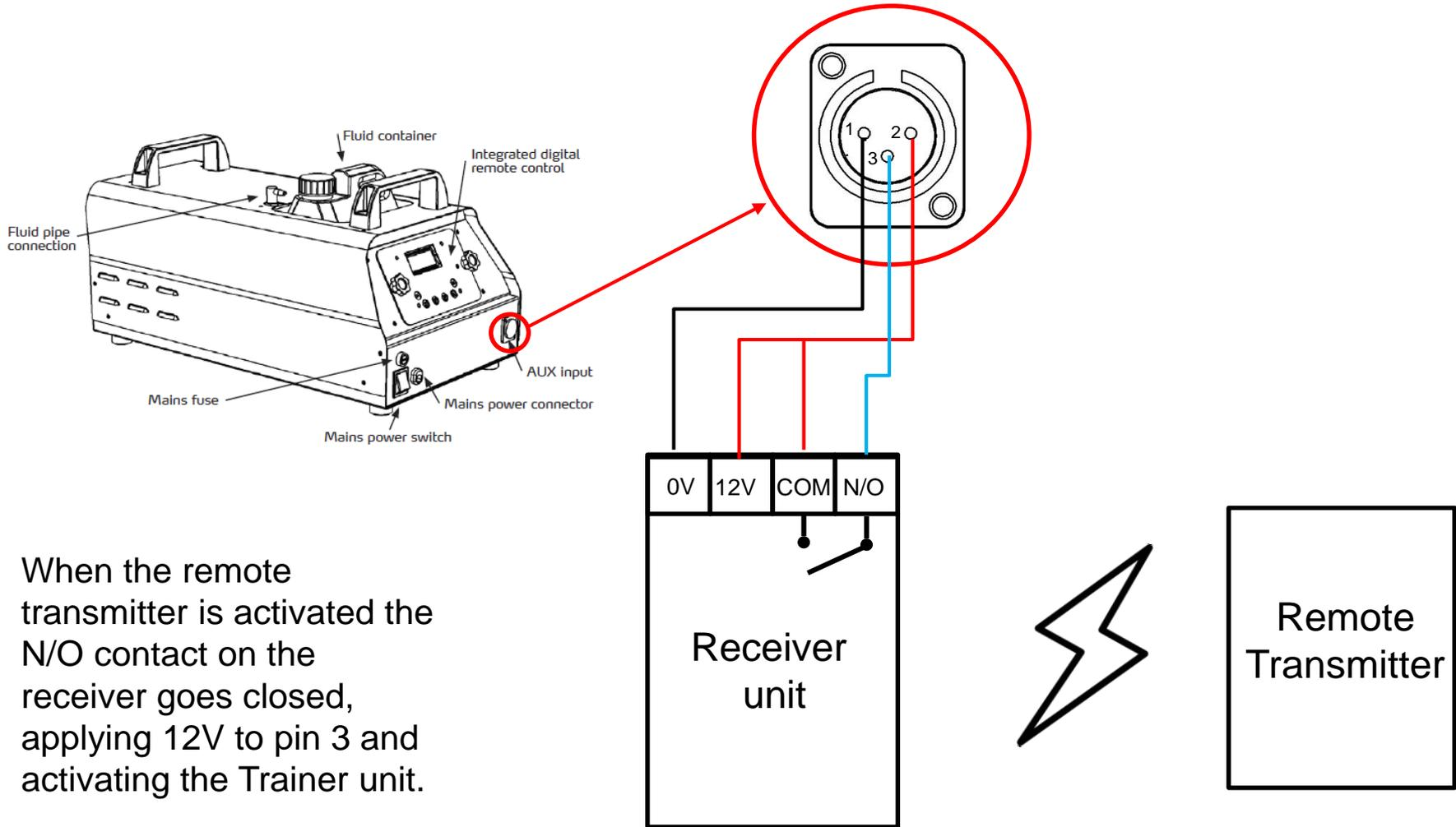
When the remote transmitter is activated the N/O contact on the receiver goes closed, applying 12V to pin 3 and activating the Trainer unit.
