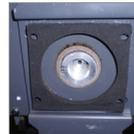
Remove the 4 x M4x10 Black Taptite Screws from the Trim Plate in front of the nozzle.
