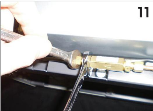
Using size 10 and 12 spanners, loosen the Brass Nut connecting the Non-Return Valve to the steel fluid pipe as shown.
