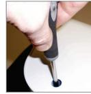
Remove the L/H side cover by removing the Hole Plugs and loosening the four screws.
