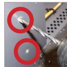
Drill out the 2 x Silver Rivets on the upper part of the vertical strap as shown, using a 3.5mm Drill bit.
