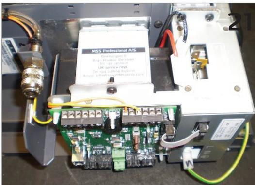
Re-connect Power Lead and power up machine. Then re-connect Battery Leads and 6-Way Connector and ensure Fluid Sensor and Fluid Bottle are correctly re-connected and installed.
