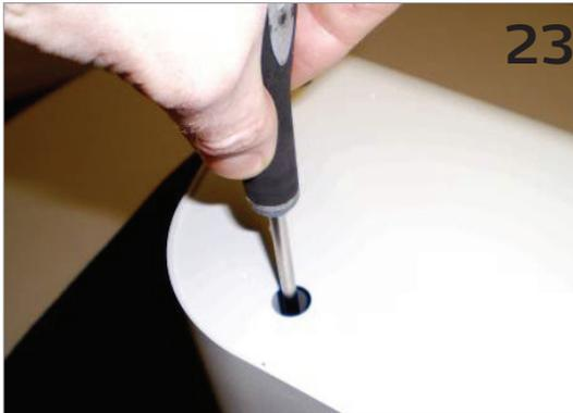
Finally, tighten the 4 x screws and replace the 4 x white hole plugs (L/H) and repeat for the 2 x screws/ hole plugs on the R/H.
