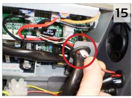
Then gently feed the white Header through the black grommet on the top of the Electronics Module as shown.
