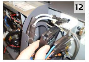
Now remove the 4 x M3 Nylocs holding the faulty Fan in place. If necessary, gently space the two upper elements of the Heat Exchanger to provide access to the upper Nyloc.
