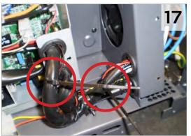
Pull the excess wire through and secure neatly to main loom using cable ties. Ensure that no part of the fan wire is protruding where it may be cut or damaged when the side covers are replaced.
