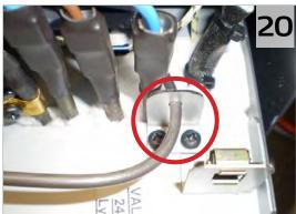
Re-attach the small metal bracket using the 2 x M4x10 Black Taptite Screws as shown.
