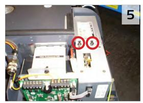
Now remove the 2 x M4x10 Black Pozzi Screws and remove the silver spacer on the electronics module as shown. This will allow you to slide the Electronics Module away from the main chassis to allow access to the screws holding the Electronics Top Cover in place.
