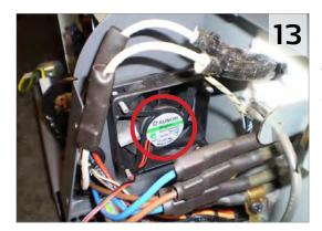
Place your replacement Fan onto the mounting posts ensuring that the label on the center of the fan is facing outwards and that the wire is orientated as shown.
