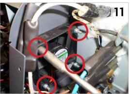
Now remove the 4 x M3 Nylocs holding the faulty Fan in place. If necessary, gently space the two upper elements of the Heat Exchanger to provide access to the upper Nyloc.
