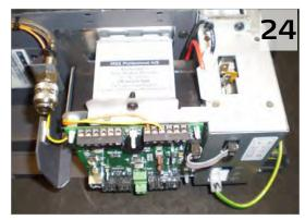
Re-connect Power Lead and power up machine. Then re-connect Battery Leads and 6-Way Connector and ensure Fluid Sensor and Fluid Bottle are correctly reconnected and installed.
