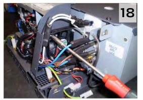
Now secure the replacement fan to the 4 mounting posts using the 4 x M3 Nylocs removed earlier.
