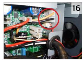
Now connect the Header onto the PCB as shown, ensuring that the connection is secure and covering all 3 pins.
