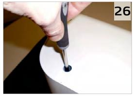
Slide L/H and R/H covers back into place ensuring tabs on inside of each cover are correctly aligned with the central vertical strap. Also, ensure that the earth leads are reconnected on both covers. Finally, tighten the 4 x screws and replace the 4 x white hole plugs (L/H) and repeat for the 2 x screws/hole plugs on the R/H.
