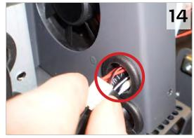
Gently feed the white Header on the end of the fan wire through the 'upper' black grommet as shown.
